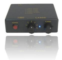
LA800 is AOR's new (receive only) outdoor shielded loop antenna for reception between 10kHz and 500MHz, divided into 6 bands. Loop element diameter: 80cm. A shielded loop antenna has the advantage, over non shielded ones, to be very robust against local noise from electrical devices.
